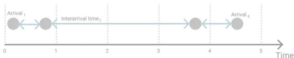
Figure 1: Illustration of a Poisson Process. Notice in here there are four arrivals up to time five, and three waiting times between arrivals.
